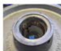
INTEGRAL (15", 16", 18") Image shows area where seal fits
